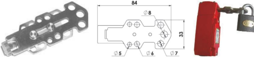
Maintenance Lock Out Actuator. Fits to IDEM Tongue Switches. Manufactured in Stainless Steel. Fits to switch aperture during maintenance and provides multiple padlock holes. Shown fitted to KM Switch (padlock not included).
